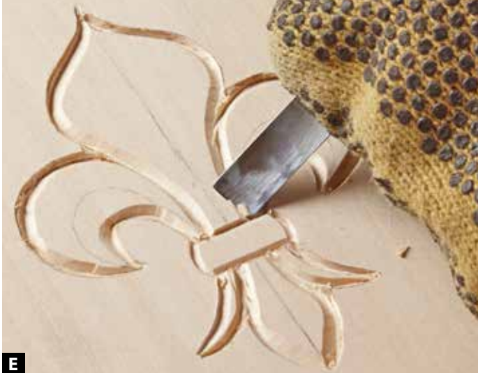
E Use a #3 gouge to pare away material above and below the crossband to make the petals taper down to, and appear to go under, the crossband.
