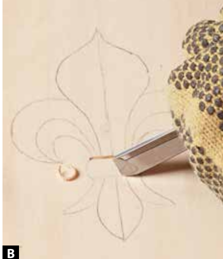
B When using the V-parting tool, hold it so the outside face of the blade—closest to the outside of the pattern—stands perpendicular to the worksurface.
