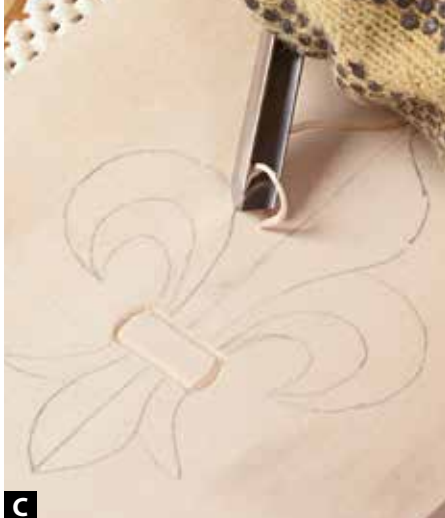
C As you carve from the top of the fleur-de-lis toward the crossband using the V-parting tool, approach the band slowly to avoid cutting into it.
